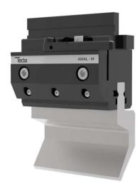
Manual clamping system for upper tools by means of a comfortable ergonomic lever. Automatic alignment of punches with safety pins and with click system
